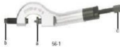
a) Chisel b) Threaded anvil with spanner flats c) Forcing screw
