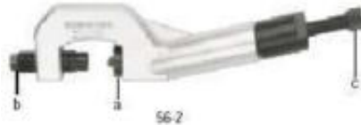
a) Chisel b) Threaded anvil with spanner flats c) Forcing screw
